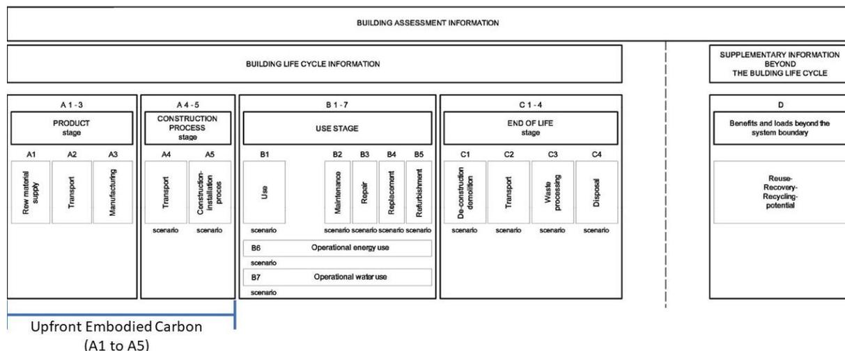
Figure 2-1: EN 15978 Building Life Cycle Assessment (LCA) Stages
